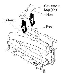
Figure 20 - Installing Crossover Log (#4)
